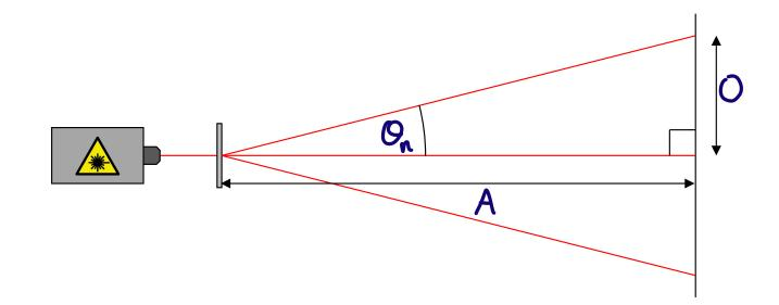
A laser (with a power less than 1 mW) is securely clamped, pointing at a diffraction grating held in position just in front of it. A piece of paper attached to a vertical surface acts as a screen.
