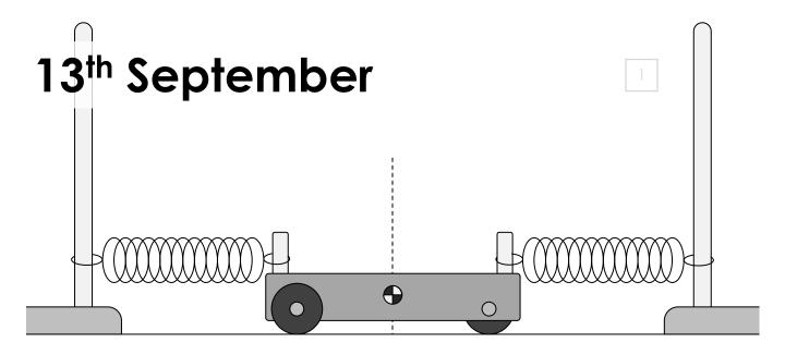
1. A wooden trolley is connected to two identical springs which are attached to two retort stands held firmly in place, as shown above.
