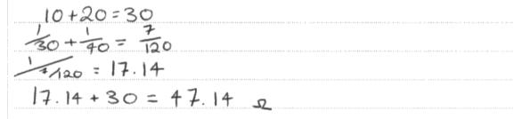
The following student added the reciprocals of the correct resistors for the parallel part of the circuit but forgot to then find the reciprocal of that answer. This was a common error.
