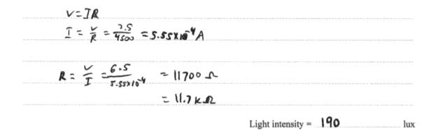
The following student attempted to use the principle of a potential divider circuit but made the common error of thinking that the voltmeter was across the LDR and not the resistor.  $R_2$  refers to the LDR resistance, and hence the pd on the left hand side of the equation should have been 6.5V.
