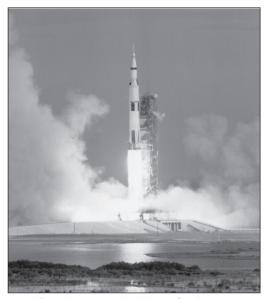
Rocket physics, in the most basic sense, involves the application of Newton's laws to a system with variable mass. A rocket has variable mass because its mass decreases over time, as a result of its fuel (propellant) burning off.
