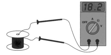
The diameter of the wire was measured as  $0.27 \text{ mm} \pm 0.01 \text{ mm}$ . The length of the wire was measured as  $1.25 \text{ m} \pm 0.05 \text{ m}$ .
