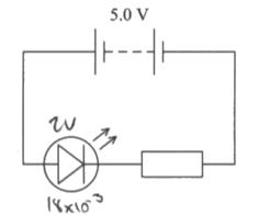
To be lit to normal brightness the current through the LED must be 18 mA.
